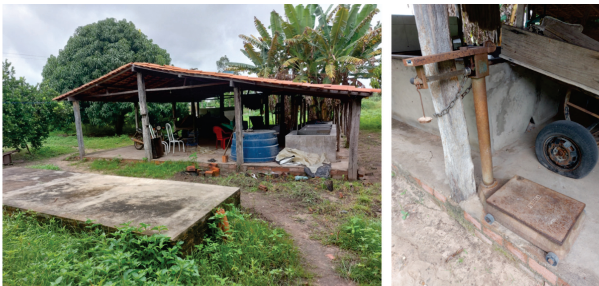
Figure 8 – Slab for drying cassava starch (a), left, and mechanical scale for weighing (b)
