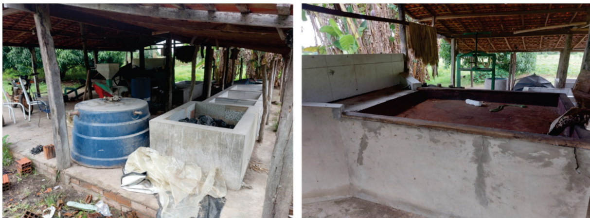
Figure 7 – Concrete tanks with stakes for washing cassava (a), left, and oven for roasting cassava flour and cooking tapioca (b)
